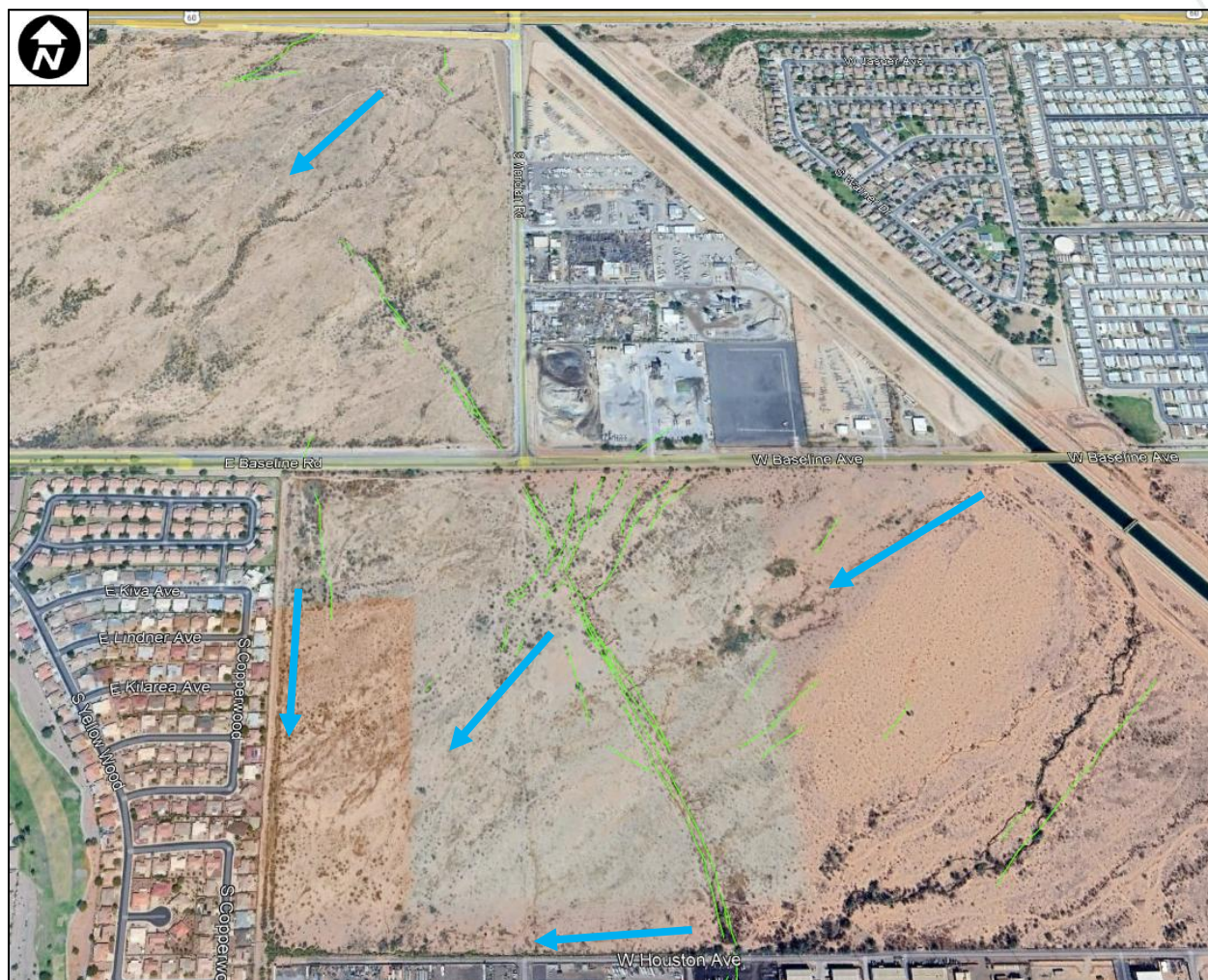
Figure 3-28. US 60 to Houston Avenue Drainage Patterns
