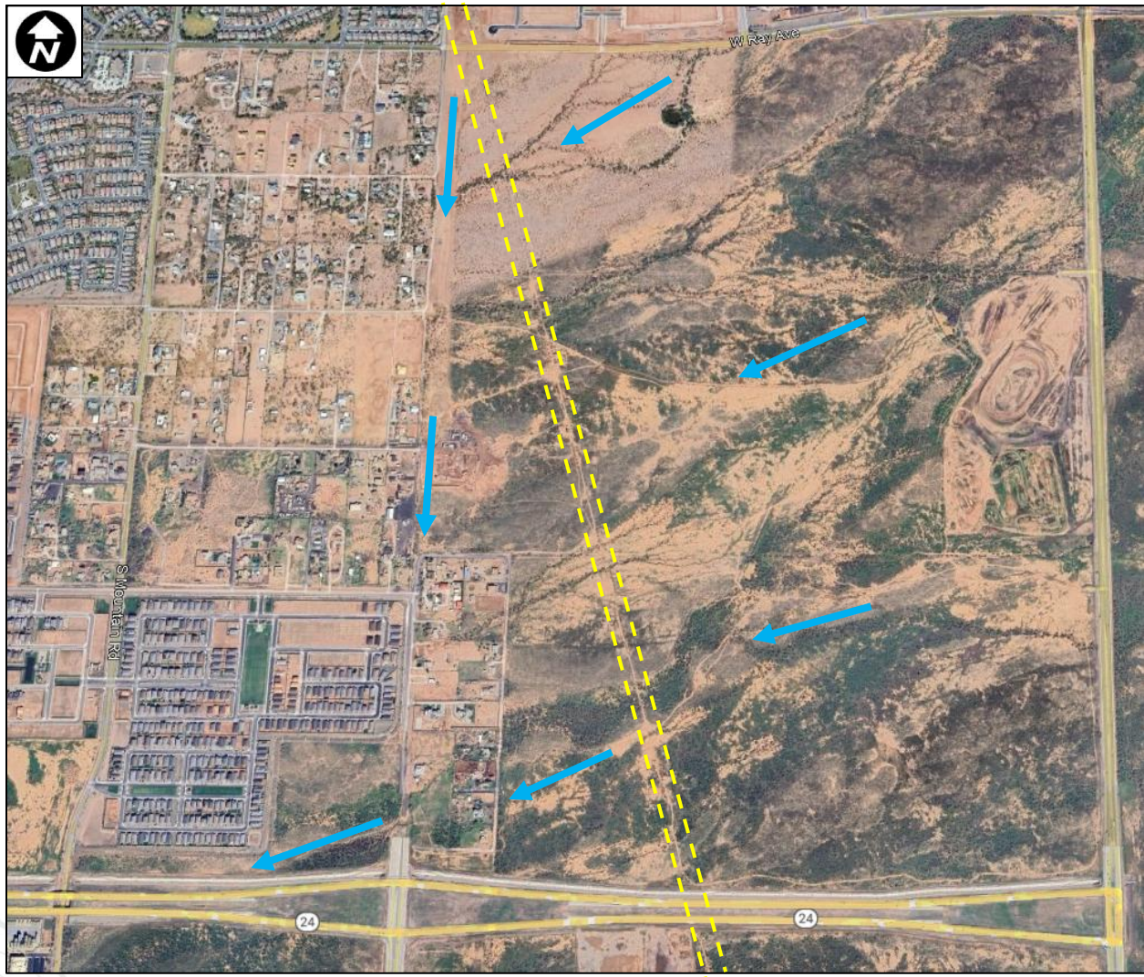
Figure 3-33. Ray Road to SR 24 Drainage Patterns
