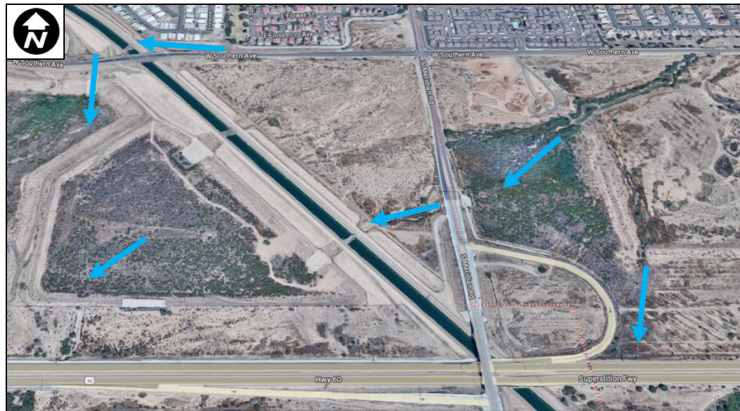
Figure 3-27. Southern Avenue to US 60 Drainage Patterns
