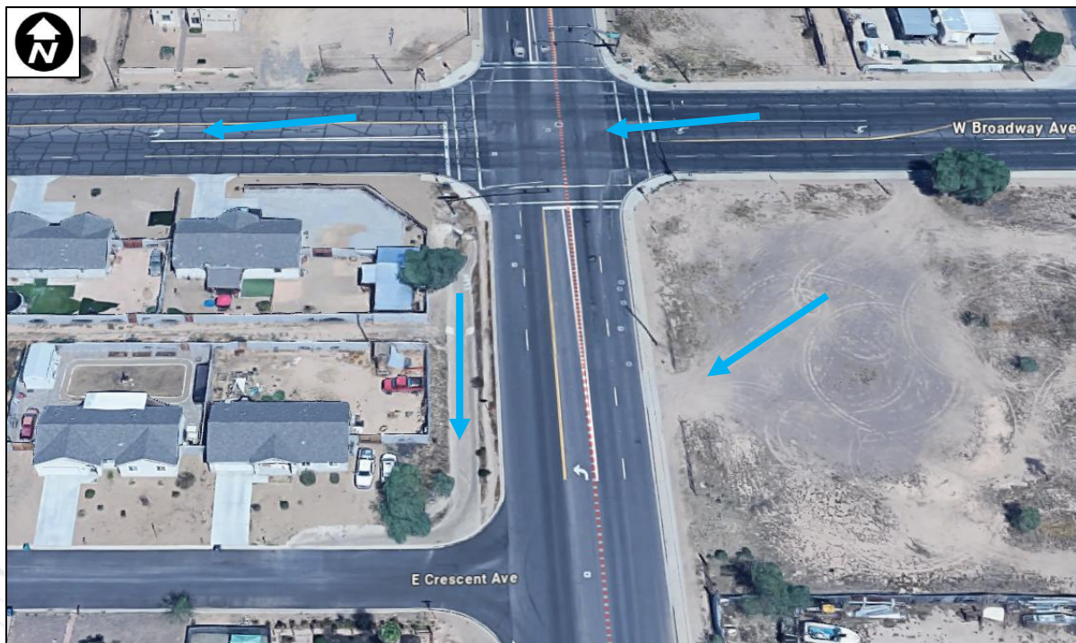
Figure 3-26. Broadway Ave & Crescent Ave Drainage Patterns
